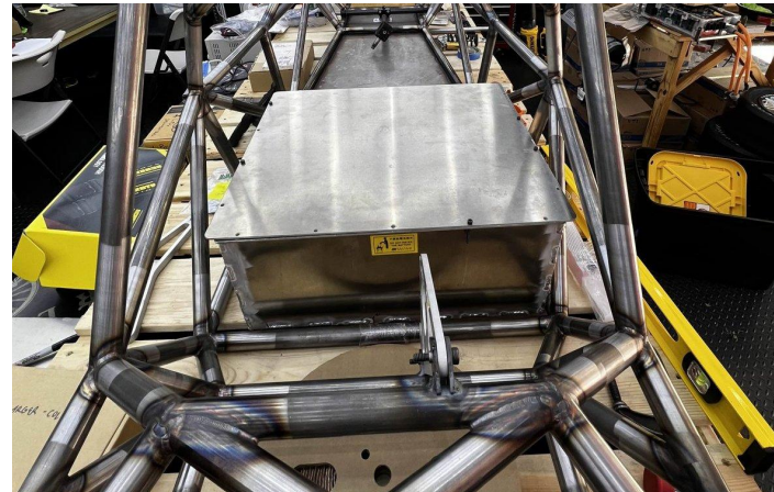
3 · Welded enclosure in the car's frame
